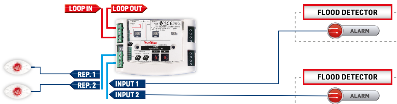
Module TFM20 - Application scheme
