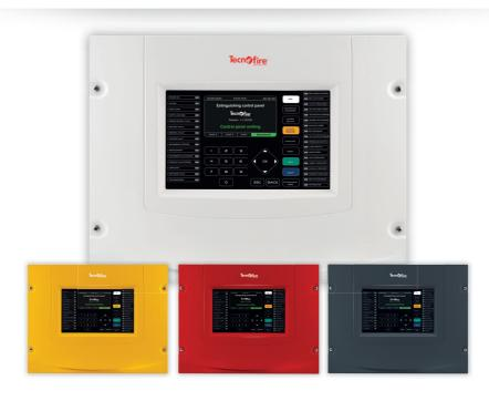
Addressable fire detection and extinguishing control panel. The characteristics listed refer to the TSA1 EXTENDED set-up. Equipped with a detection loop and an Extinguish Device Unit (EDU). The detection loop can handle up to 199 detectors, 99 modules and 9 TSM1 modules (peripheral EDU extinguishing channels).
